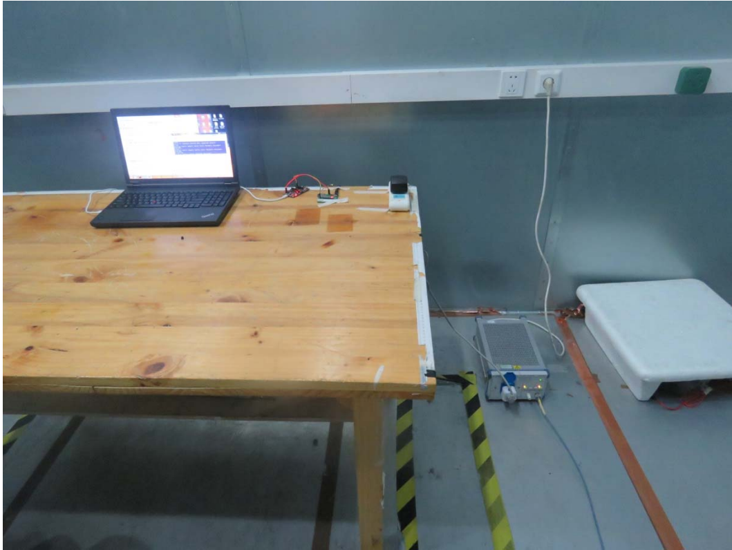
Picture 3 Conducted Emission Test Setup
