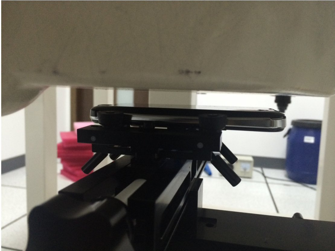
Band850, Band1900, WCDMA Band II and WIFI Test Setup Body Back with gap 10mm
