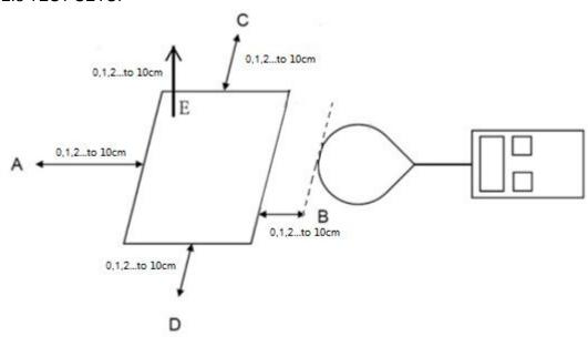
Remark: The E300 probe antenna diameter is 11.5cm.
