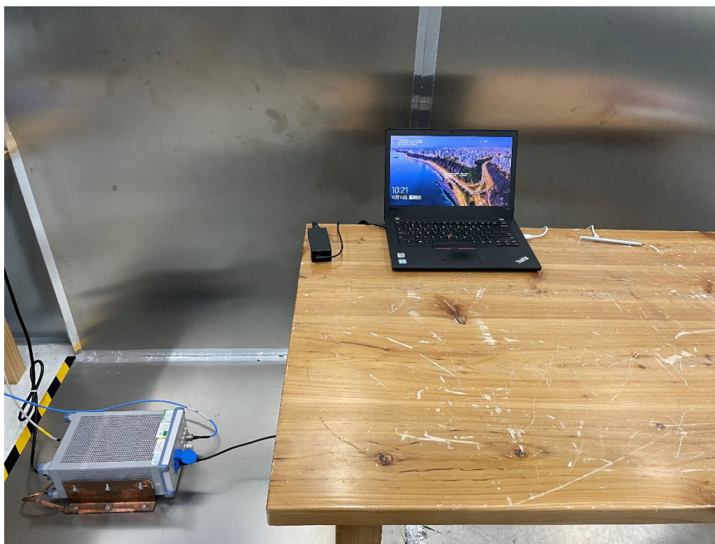
Photograph 4: Set-up for RF Exposure
