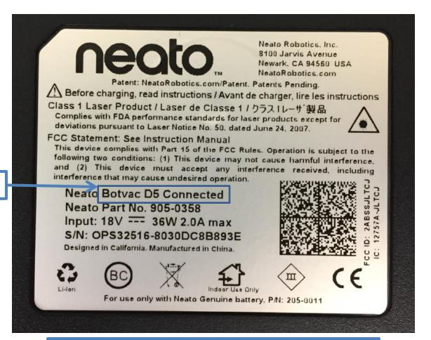
Note: Label attached via permanent adhesive (acrylic-based), printed on mylar stock resinbased ink
