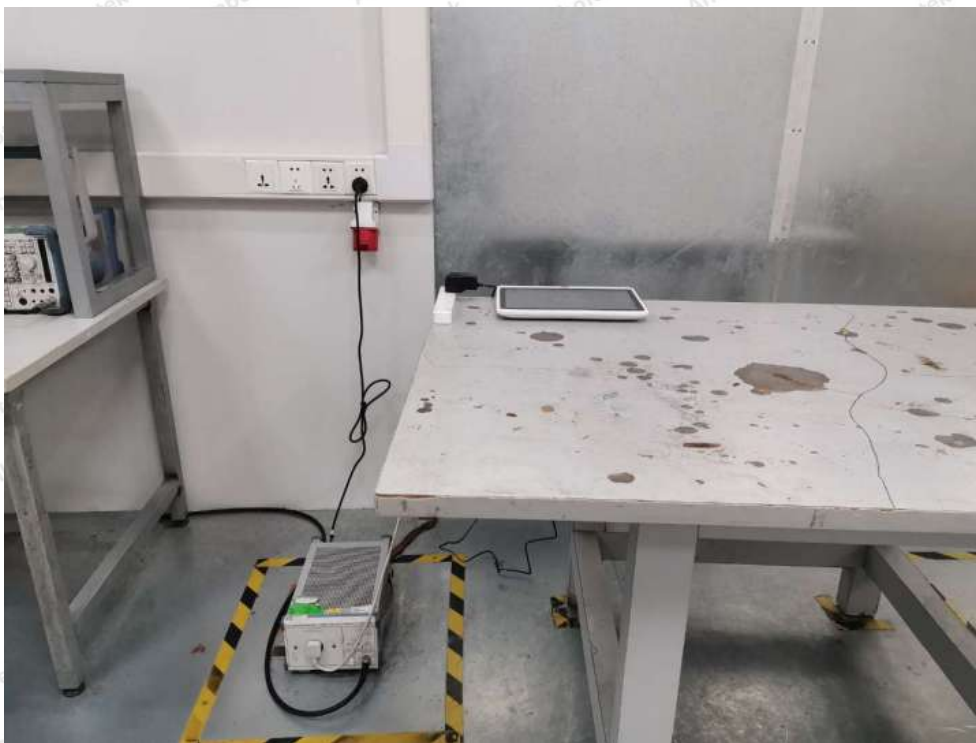
Photo of Power Line Conducted Emission Test
