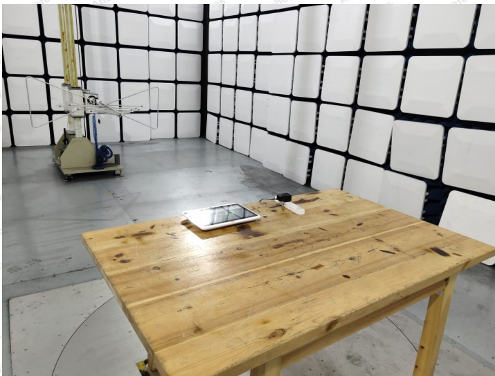
Photo of Radiation Emission Test
