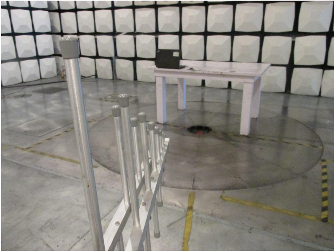
Radiated Emission Test setup photos
