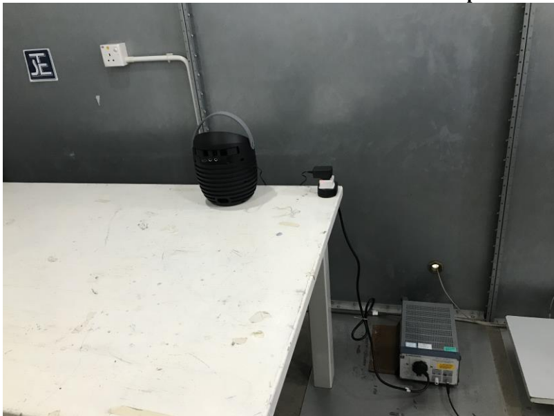
Measurement of Conducted Emission Test Set Up
