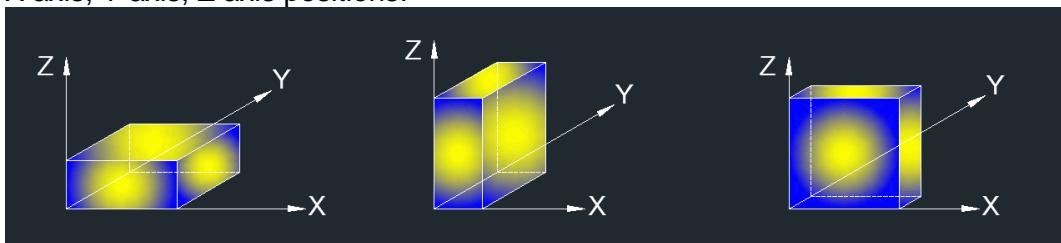
Note: For all radiated test, EUT in one orthogonal axis (X axis) emissions had been tested and recorded in the report.
