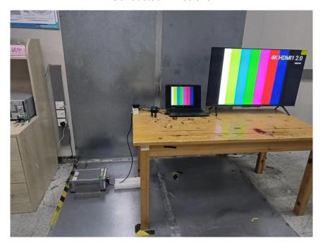
Radiated Emissions From 30MHz-1000MHz
