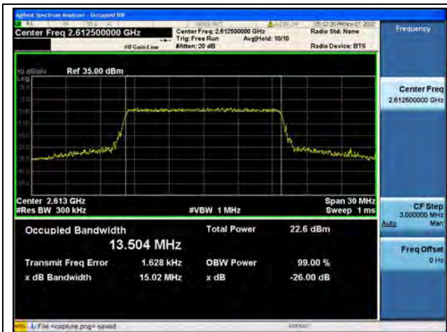
Band38 / 15MHz / QPSK / High CH
