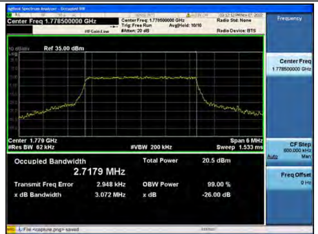
Band66 / 3MHz / QPSK/ High CH
