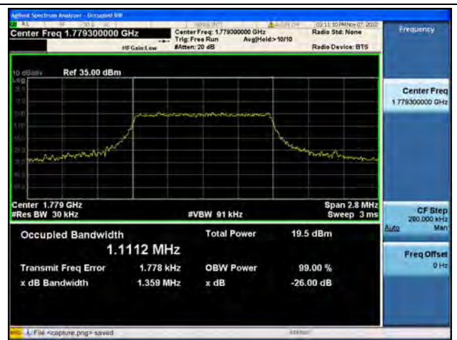
Band66 / 1.4MHz / 16QAM/ High CH
