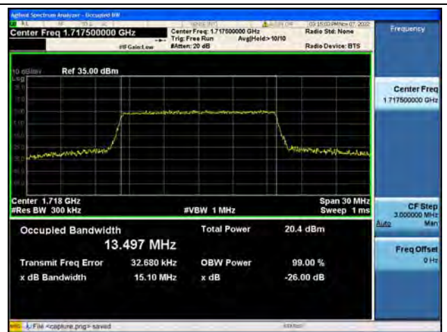
Band66 / 15MHz / 16QAM/ Low CH
