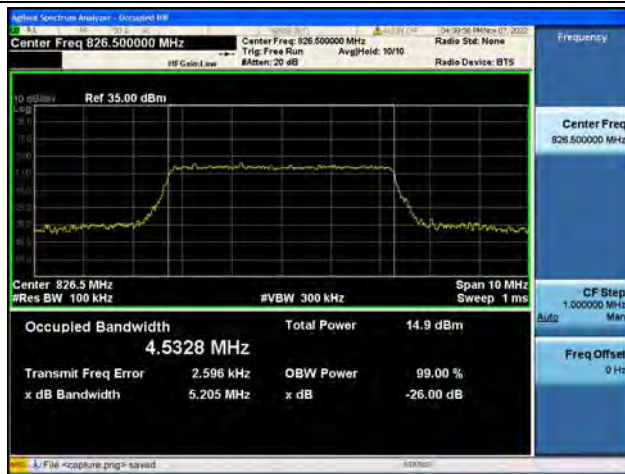
Band26Part22 / 5MHz / 64QAM/ Low CH
