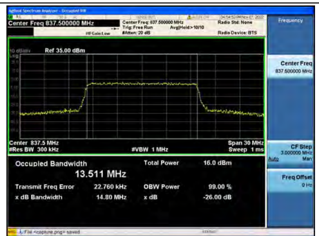
Band19 / 15MHz / 16QAM/ Low CH
