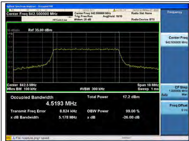
Band19 / 5MHz / QPSK/ High CH
