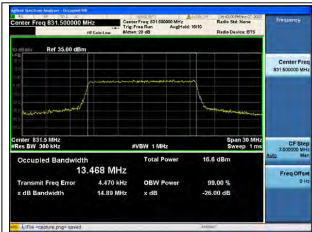
Band26Part22 / 15MHz / QPSK/ Low CH
