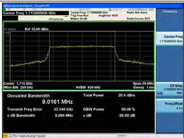
Band66 / 10MHz / 16QAM/ Low CH
