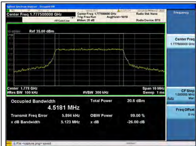
Band66 / 5MHz / QPSK/ High CH
