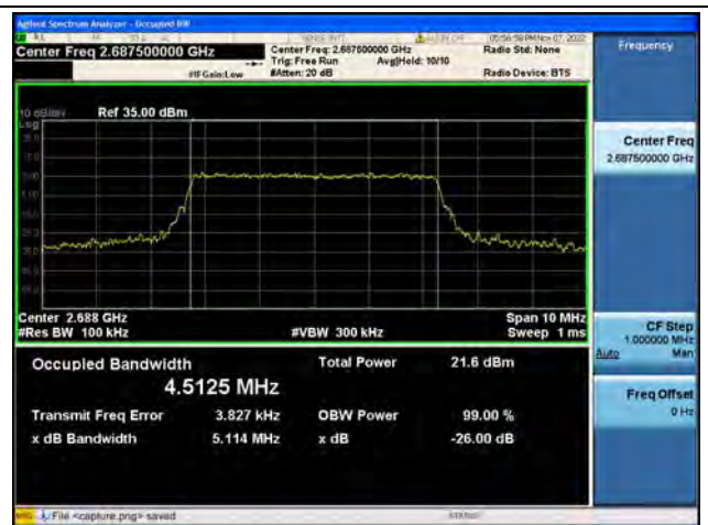
Band41 / 5MHz / 16QAM/ High CH
