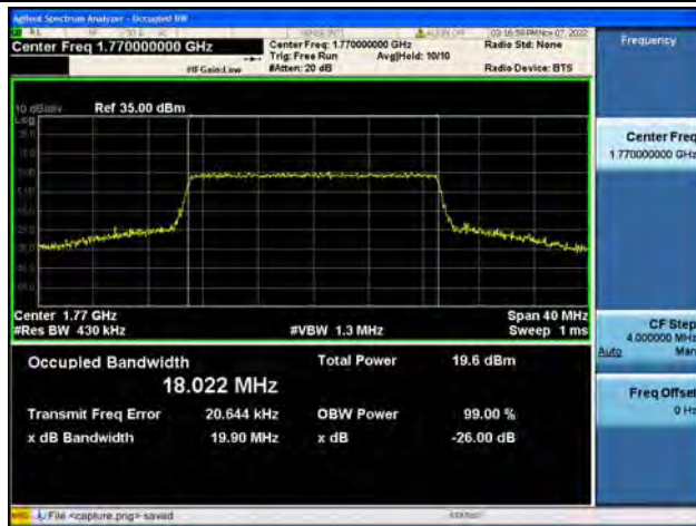
Band66 / 20MHz / 16QAM/ High CH
