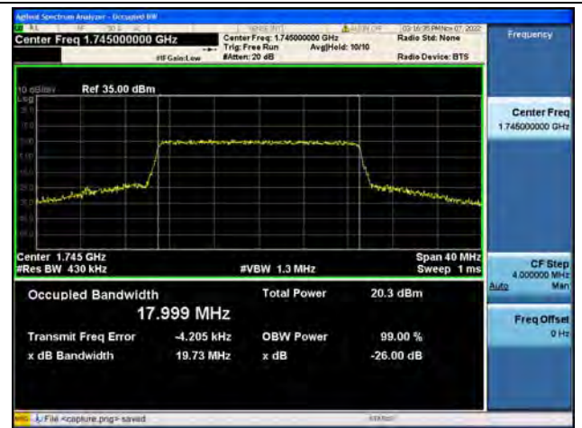
Band66 / 20MHz / 16QAM/ Mid CH
