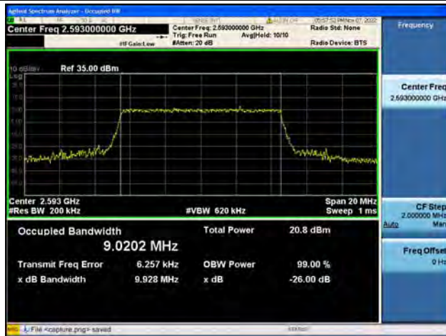
Band41 / 10MHz / 64QAM/ Mid CH
