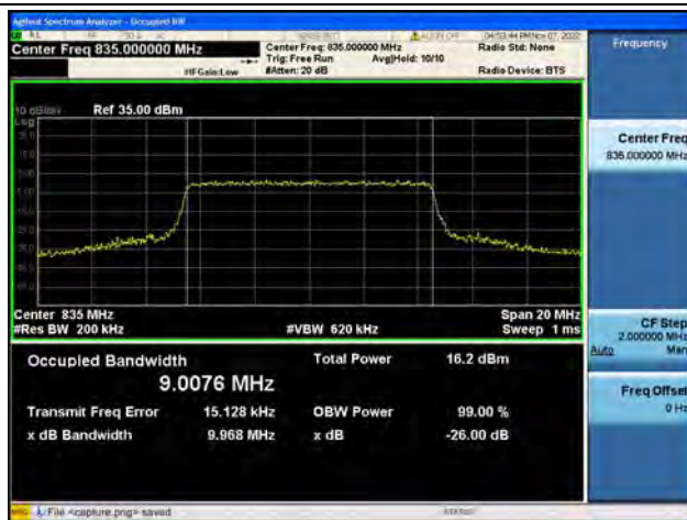
Band19 / 10MHz / 16QAM/ Low CH
