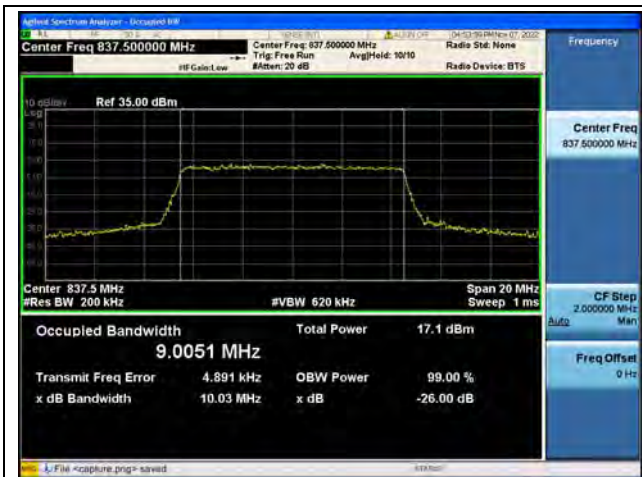
Band19 / 10MHz / QPSK/ Mid CH
