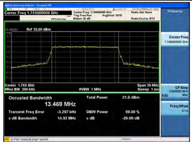
Band66 / 15MHz / QPSK/ Mid CH
