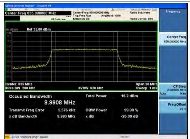
Band19 / 10MHz / 64QAM/ Low CH
