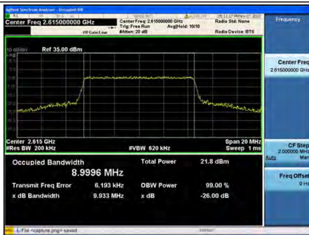
Band38 / 10MHz / 16QAM/ High CH
