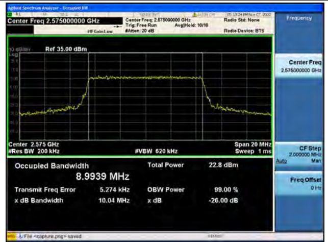
Band38 / 10MHz / QPSK/ Low CH
