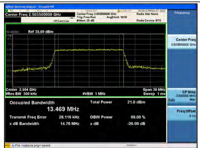
Band41 / 15MHz / 16QAM/ Low CH
