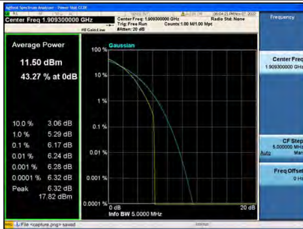
Band2 / 1.4MHz / High CH / 64QAM
