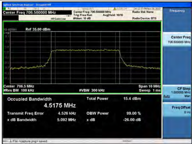
Band17 / 5MHz / 64QAM/ Low CH
