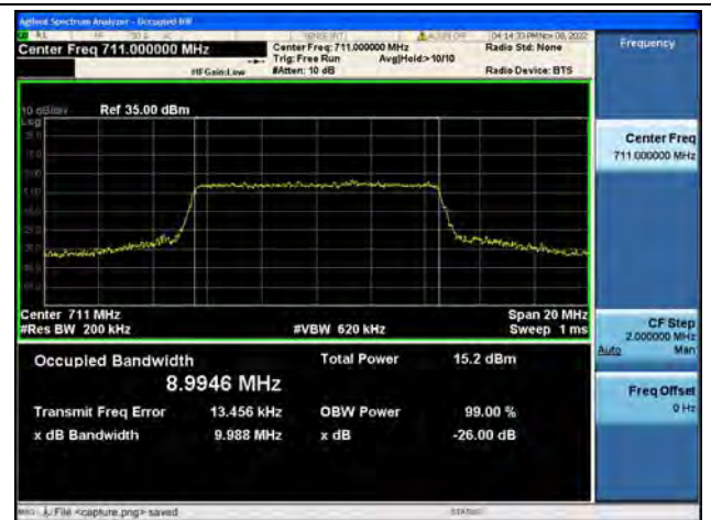
Band17 / 10MHz / 64QAM/ High CH
