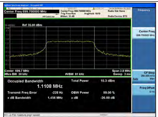
Band12 / 1.4MHz / 16QAM/ Low CH
