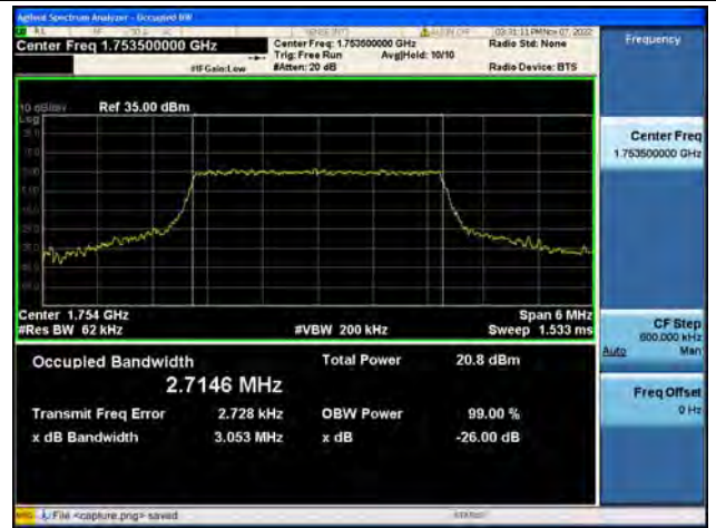
Band4 / 3MHz / QPSK/ High CH
