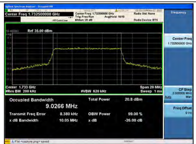
Band4 / 10MHz / 16QAM/ Mid CH
