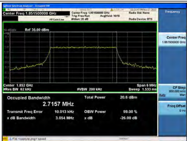
Band2 / 3MHz / 16QAM/ Low CH
