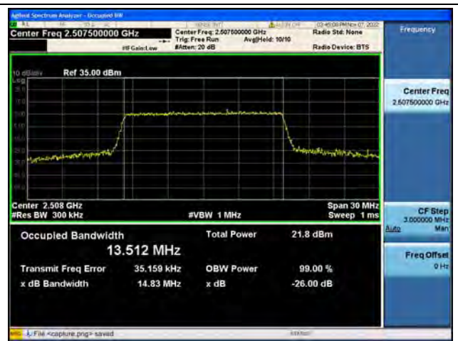
Band7 / 15MHz / 16QAM/ Low CH
