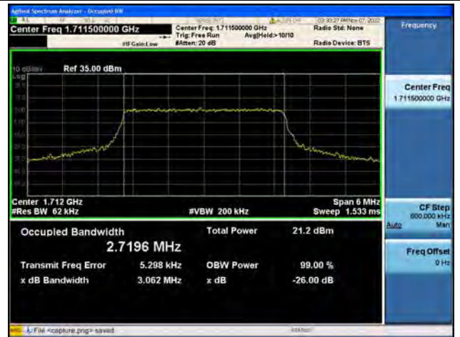
Band4 / 3MHz / QPSK/ Low CH
