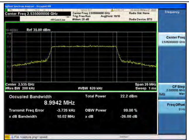
Band7 / 10MHz / 16QAM/ Mid CH
