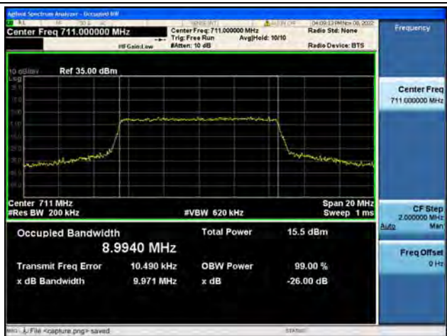
Band12 / 10MHz / 16QAM/ High CH
