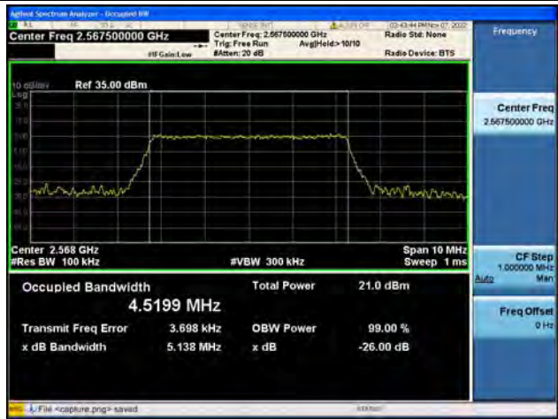
Band7 / 5MHz / 64QAM/ High CH
