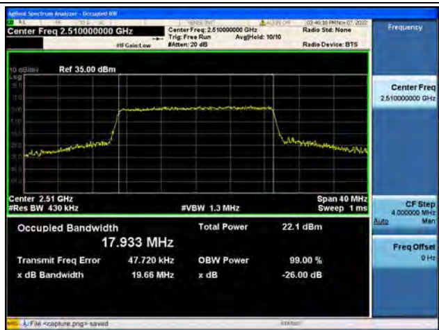
Band7 / 20MHz / 16QAM/ Low CH
