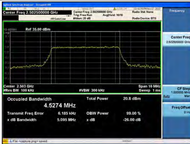
Band7 / 5MHz / 64QAM/ Low CH
