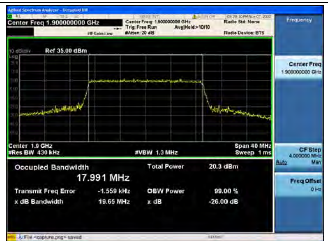
Band2 / 20MHz / 64QAM/ High CH
