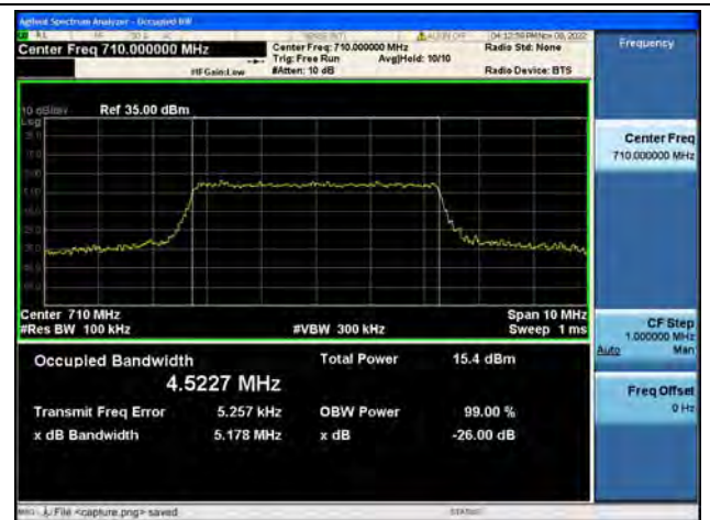
Band17 / 5MHz / 64QAM/ Mid CH
