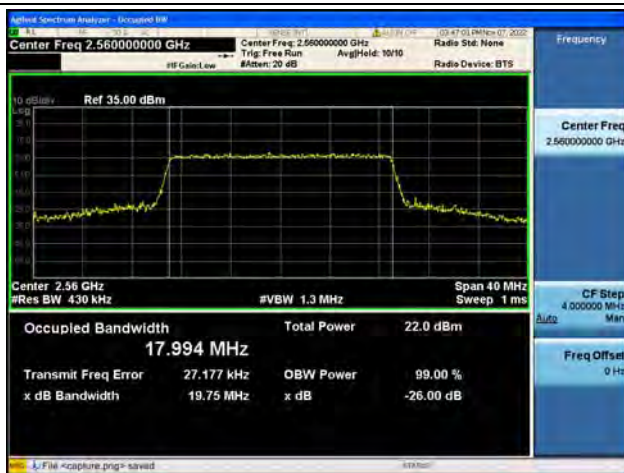
Band7 / 20MHz / 16QAM/ High CH
