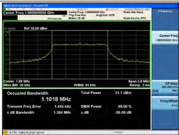
Band2 / 1.4MHz / 16QAM/ Mid CH
