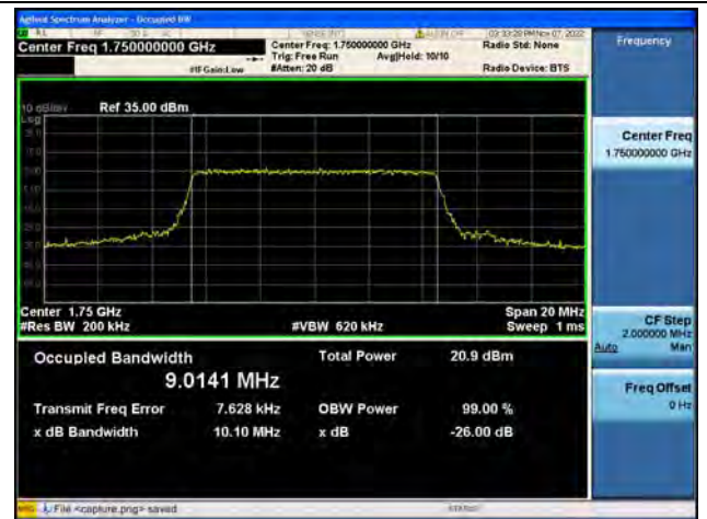
Band4 / 10MHz / QPSK/ High CH
