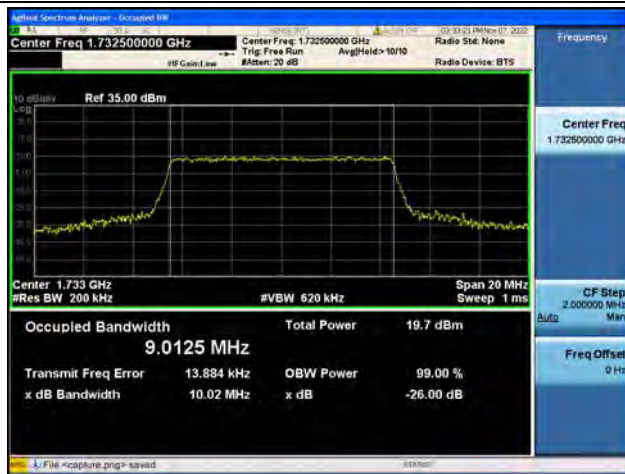
Band4 / 10MHz / 64QAM/ Mid CH
