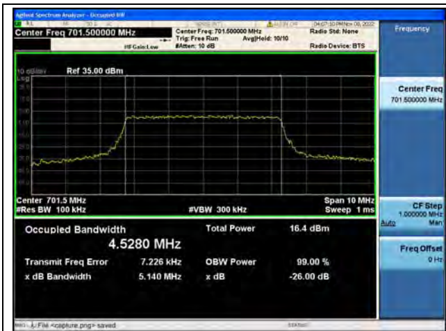
Band12 / 5MHz / QPSK/ Low CH
