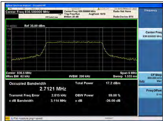
Band5 / 3MHz / QPSK/ Mid CH
