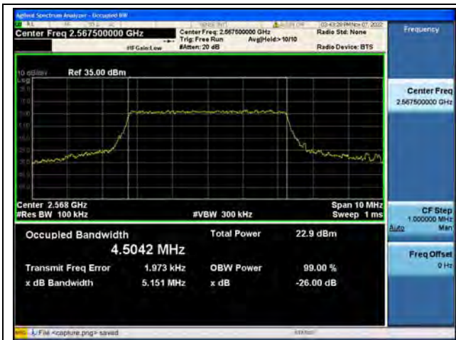
Band7 / 5MHz / QPSK/ High CH
