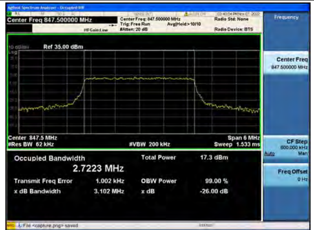
Band5 / 3MHz / QPSK/ High CH
