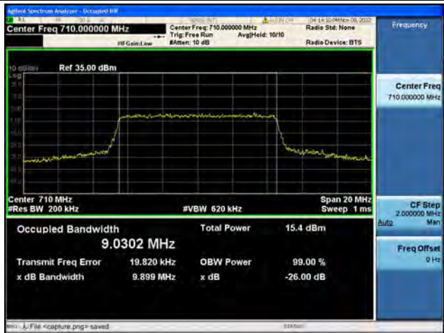
Band17 / 10MHz / 64QAM/ Mid CH
