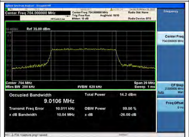
Band12 / 10MHz / 64QAM/ Low CH
