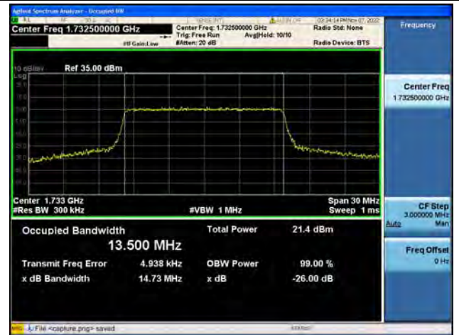
Band4 / 15MHz / QPSK/ Mid CH
