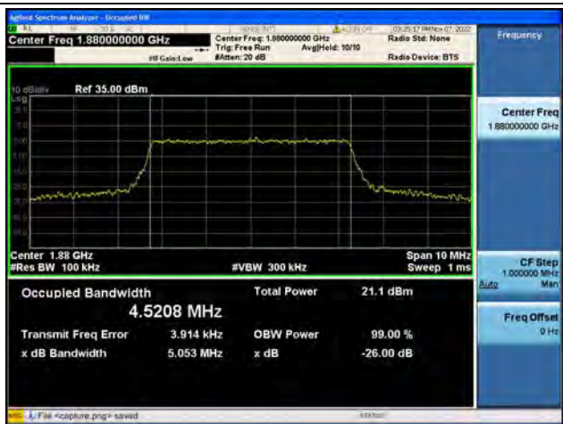
Band2 / 5MHz / 16QAM/ Mid CH
