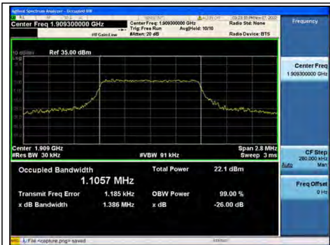
Band2 / 1.4MHz / QPSK/ High CH
