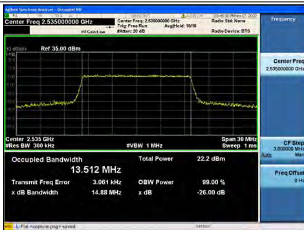
Band7 / 15MHz / 16QAM/ Mid CH
