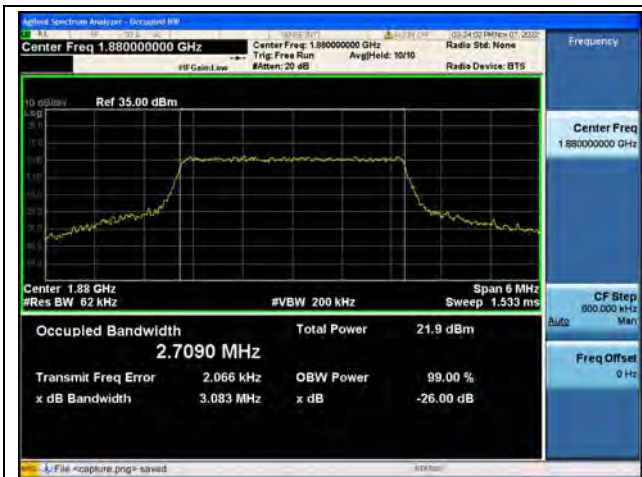
Band2 / 3MHz / QPSK/ Mid CH
