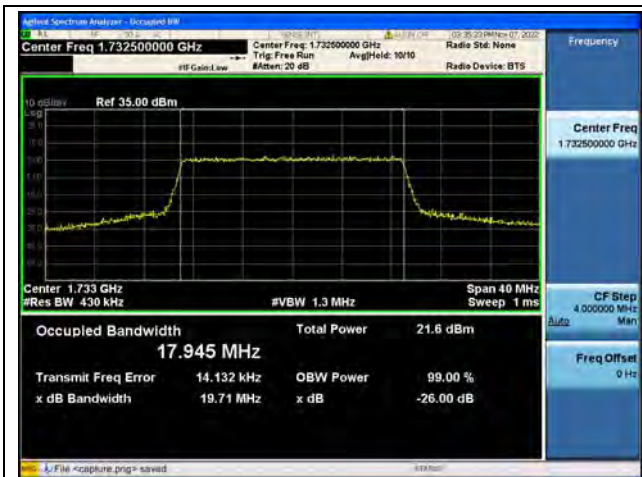
Band4 / 20MHz / QPSK/ Mid CH
