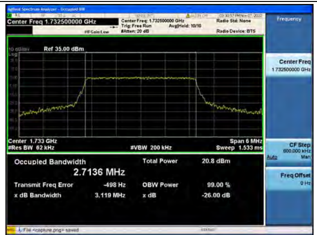
Band4 / 3MHz / 16QAM/ Mid CH
