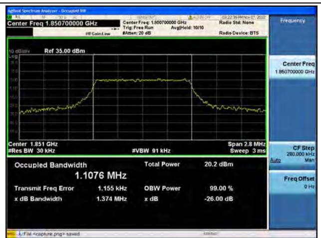
Band2 / 1.4MHz / 16QAM/ Low CH
