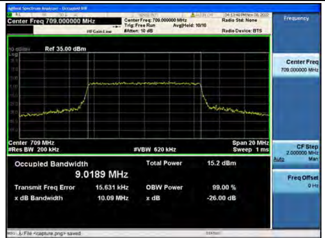
Band17 / 10MHz / 64QAM/ Low CH
