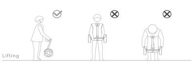
If your Mini is Power ON and in autobalance mode during carrying power output will be cut off automatically when tires are hung in the air for your safet palance mode will be recoveled automatically when plachlg Mini to the ground. Do not lift the Mini by the fender or the main frame, or your finger may be clipped or damaged in fender. Please do as shown on above.
