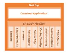
The platform efficiently manages wake and sleep states, communications, and other functions notifying the script when changes occur. Using the script capabilities, developers have full access to the device's functions without having to deal with complex embedded firmware.
