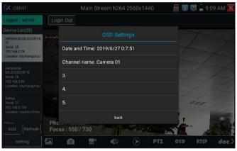
After channel selecting, you can edit the channel name, modify the display position, and switch the font size. Select "default location" in "content location" is without modification. Select "Customization" to arbitrarily adjust the channel name and display location. Click "OK" and the effects will appear. Press return key or click any area of the screen to return to the upper layer of the interface.
