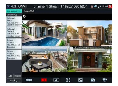
segments. It lists cameras name and IP address on the Left of screen. Tester can auto login camera and display camera image. Factory default use admin password to auto login, if you modified the password, then default use the modified password to log in.
