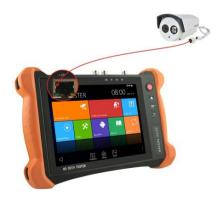
Note: 1) If the IP camera requires PoE power, then connect the IP camera to the IP tester's LAN port. The tester will supply PoE Power for the IP camera. Click the icon POE to turn the PoE Power off or on.
