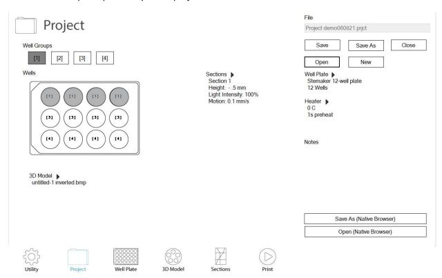
4. If heating or mixing of the bioink is needed, go to the Utility page and change the desired settings.
