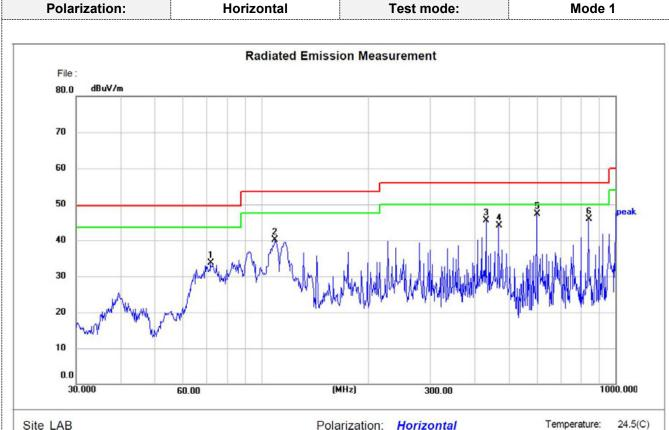
Limit: FCC Part15 RE-Class A(3m)\_30-1000MHz
