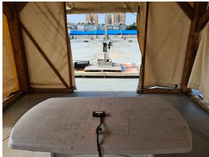
Figure 2. Radiated Emission Test, 200.0-1000.0 MHz
