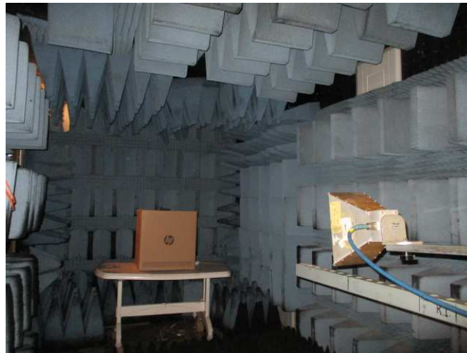
Figure 3. Radiated Emission Test, 1000.0-5000.0 MHz
