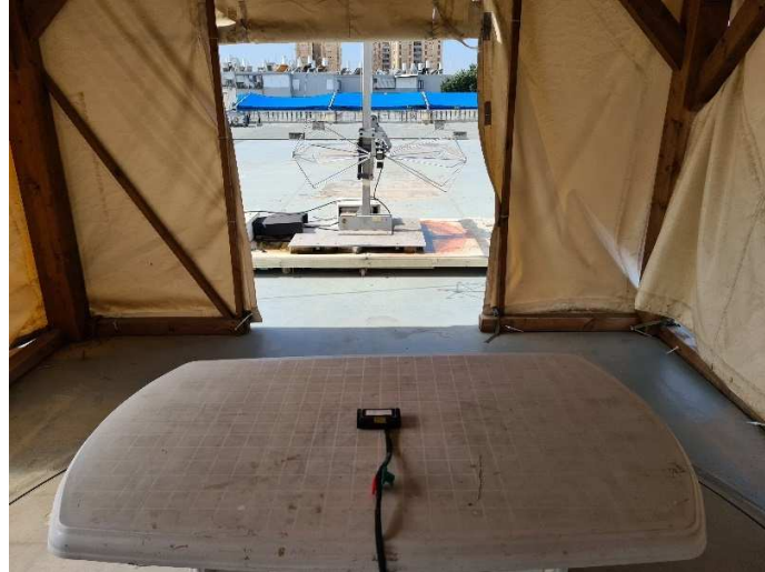
Figure 1. Radiated Emission Test, 30.0-200.0 MHz
