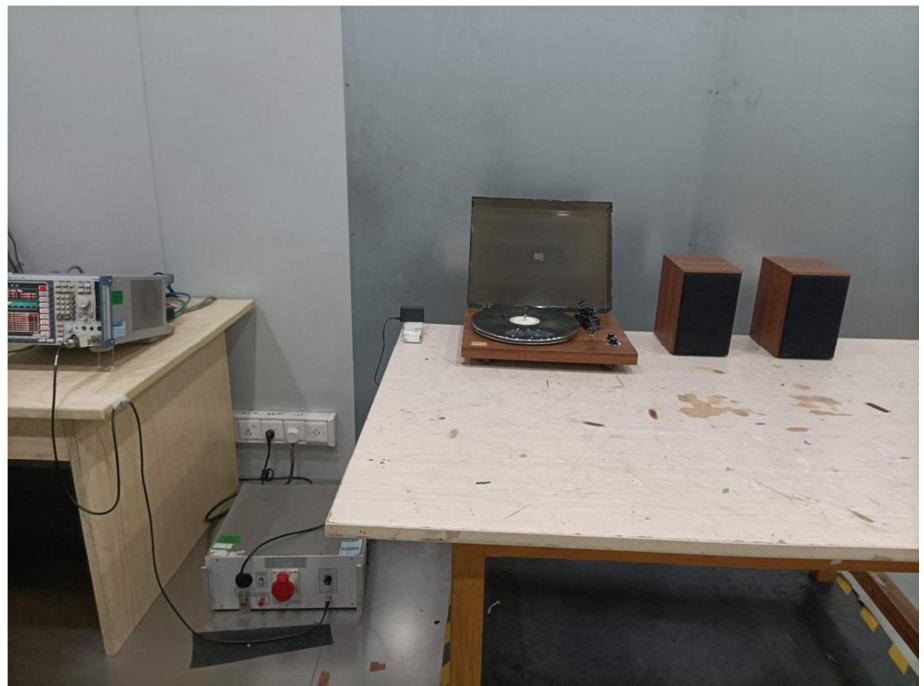
Conducted Emission Test Setup
