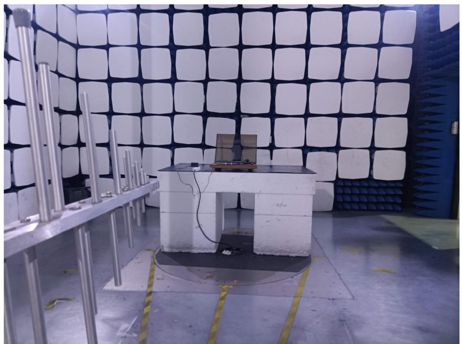
Radiation Emission Test Setup (30MHz to 1GHz)
