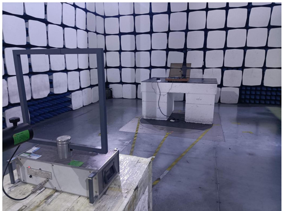
Radiation Emission Test Setup (Below 30MHz)
