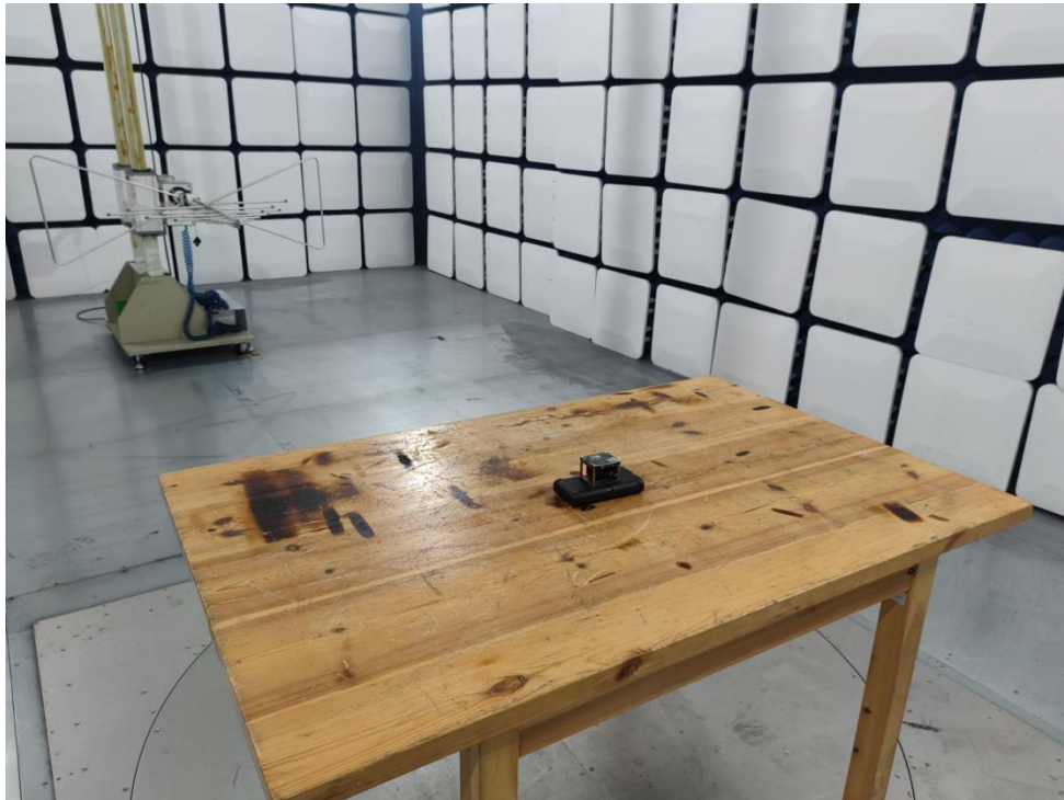
Photo of Radiation Emission Test
