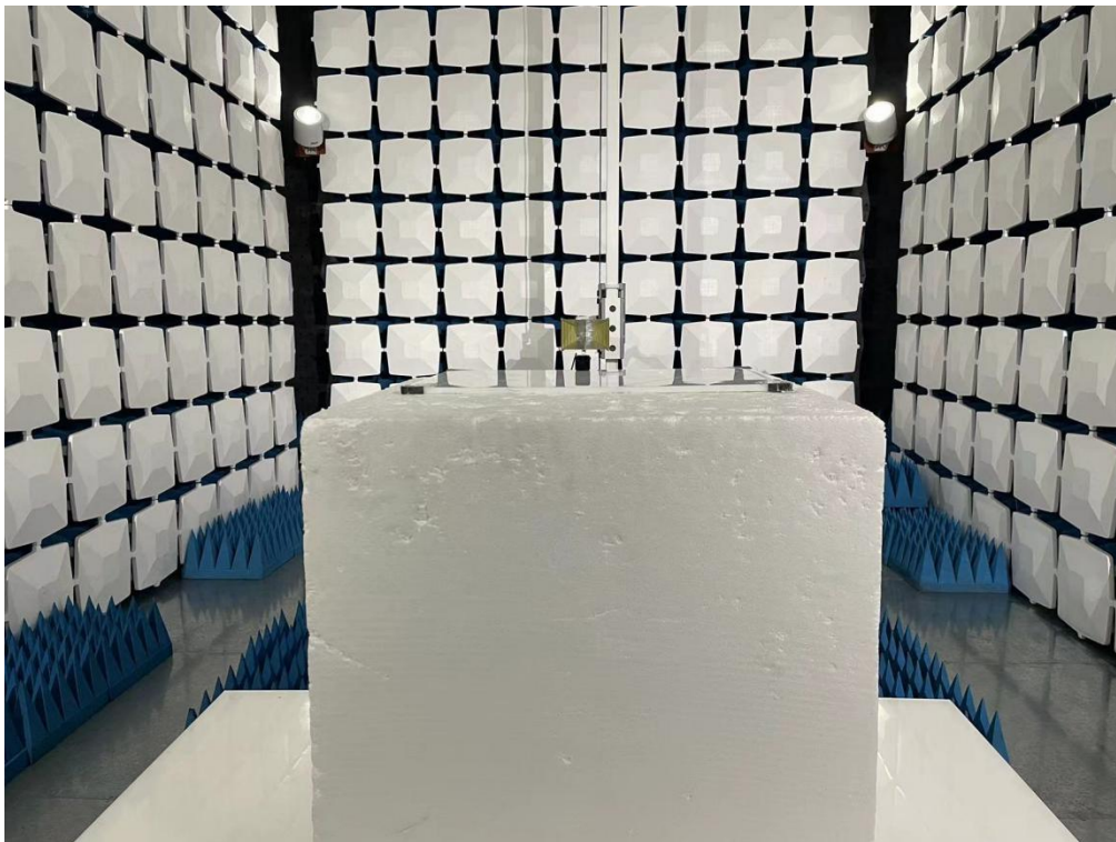
Above 1GHz for radiated emission test setup
