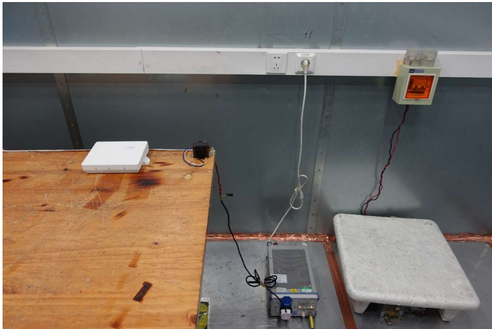
Picture 2 Conducted Emission Test Setup
