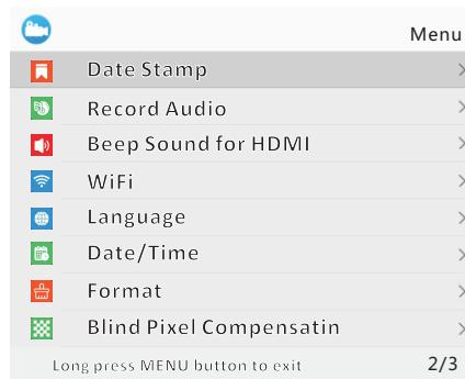
10. Record Audio: press [+ key] [- key] to move the cursor to the record audio option, and press [menu key] to enter the sub-menu, press [+ key] [- key] to select on / off recording audio, press [menu key] to confirm and exit.
