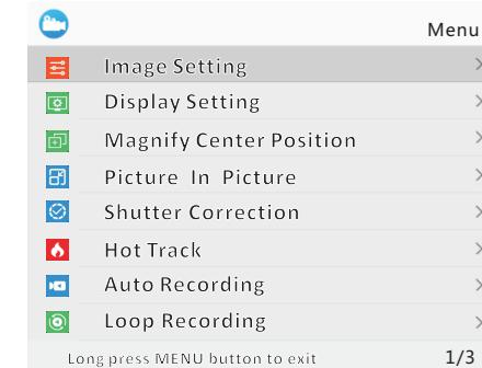
1. Image setting: press [+ key] [- key] move the cursor to the image setting option, and press [menu key] to enter the sub menu, press [menu key] to switch the contrast / brightness / sharpness / mode options, and press [+ key] [- key] to adjust
