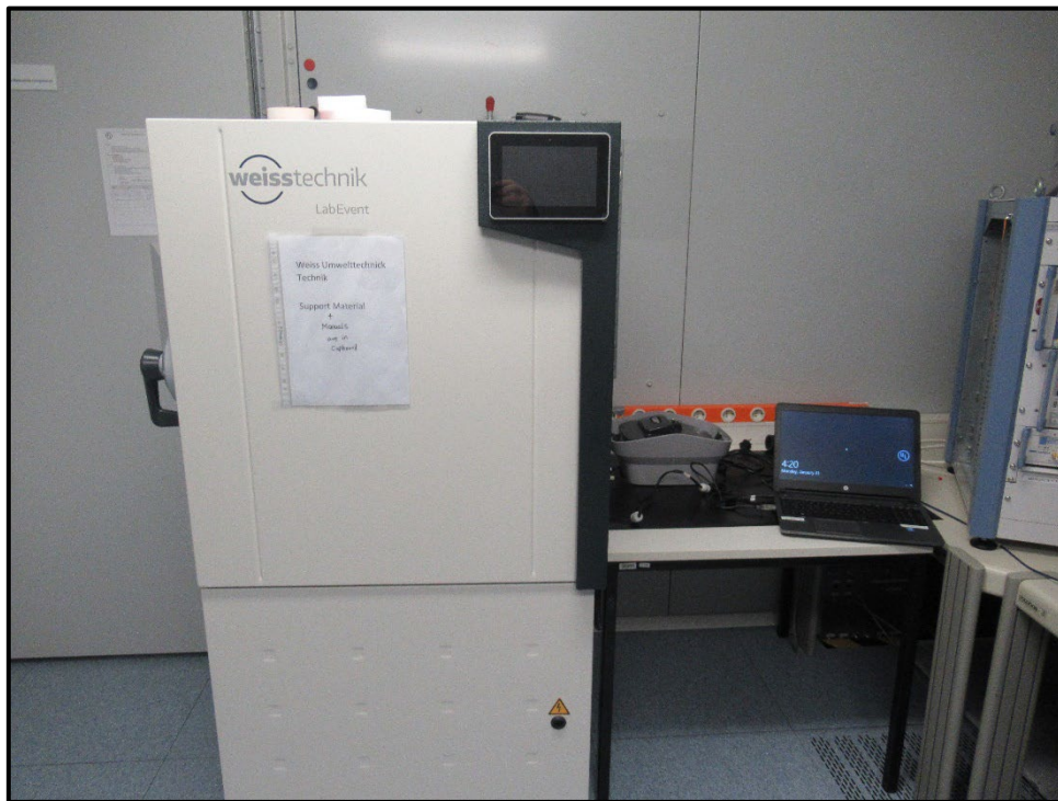
Photo 7 Conducted Test Setup-Frequency Stability + OBW measurements
