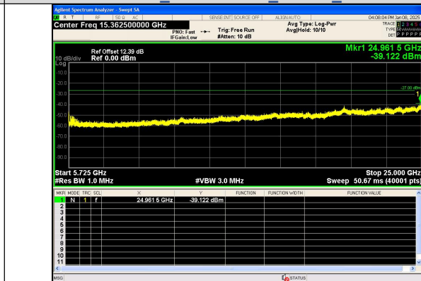
Spurious Emission:5725~25000.0 MHz IEEE 802.11n Channel 118 40MHz Antenna 0
