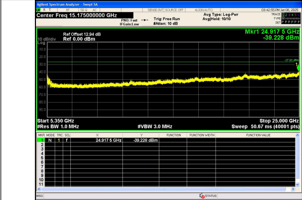
Spurious Emission:5350~25000.0 MHz IEEE 802.11n Channel 64 20MHz Antenna 0
