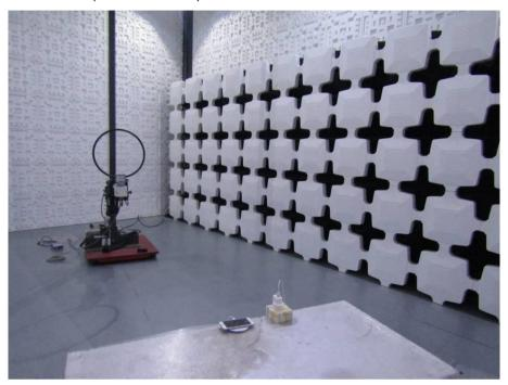
Radiated Emission (30MHz-1000MHz)
