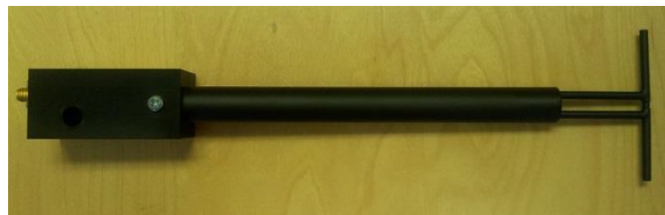
Figure 1 – MVG COMOSAR Validation Dipole
