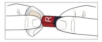
(2) Take out the new ear cap and insert the receiver against the middle of the ear cap.
