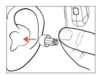
(3) Adjust the position of the receiver wire until it fits the ear.
