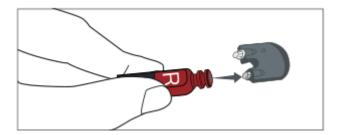
(4) Use the other needle to insert the new cerumen cap into the hearing aid, remove the tool and dispose it.
