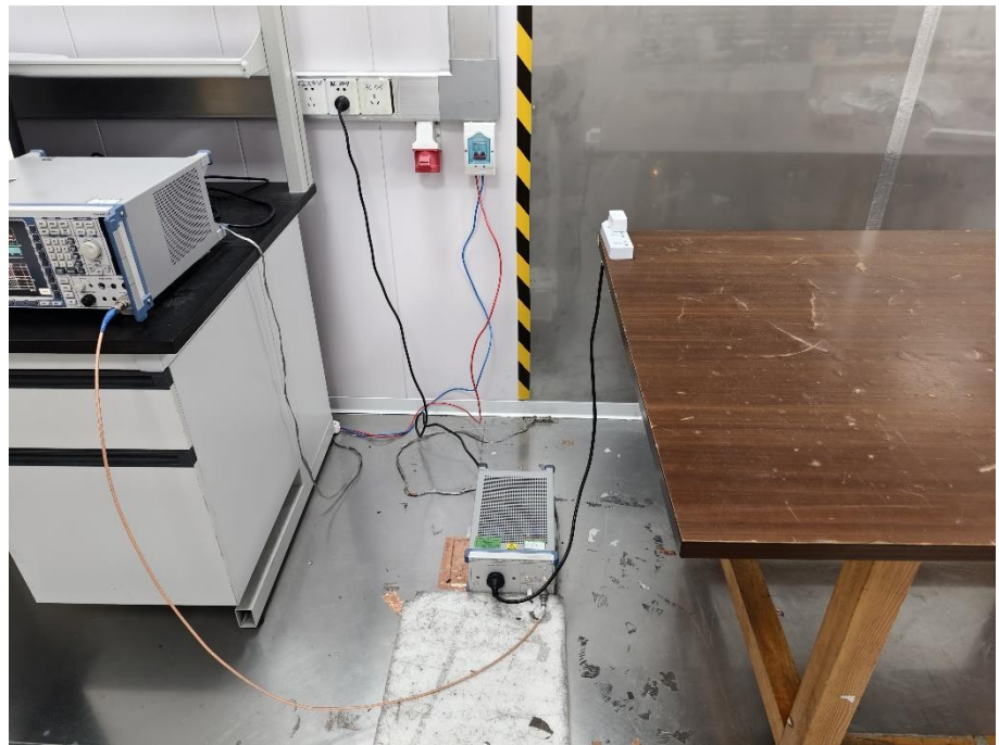
Conducted Emission Test Setup
