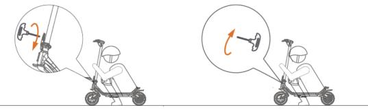
If the handlebar and its stem sway during riding, use the hexagon wrench to tighten the screws on the folding mechanism.
