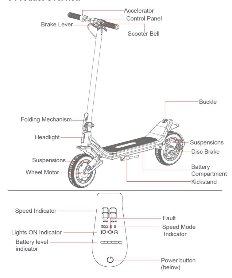
Battery level display: The power level is indicated by five power lights on the control panel. As power is consumed, the lights will change from solid to flashing, and finally turn off from up to down. When the bottom power light flashes, it indicates low power. Please recharge soon for further use. After running out of power, all lights will turn off, and the scooter will coast until it comes to a complete stop.
