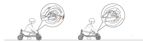
If the brake is too tight, use the hexagon wrench to loosen the screws on the caliper, and slightly send back the brake cable to shorten the exposed length, then tighten the screws. If the brake is too loose, loosen the screws, and slightly pull out the brake cable to lengthen the exposed length, then tighten the screws.
