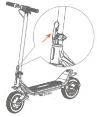
3.Use the hex wrench in the packaging box to lock the screws on both Sides.
