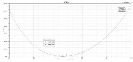
Center frequency impedance: 50 ohms @ 2.438GHz
