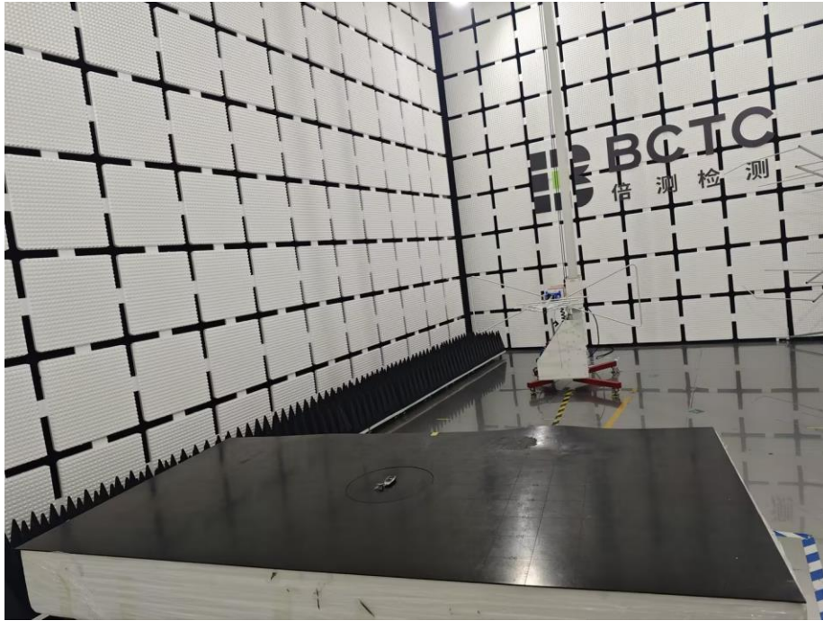
Spurious Emission Test Setup (Above 1GHz)
