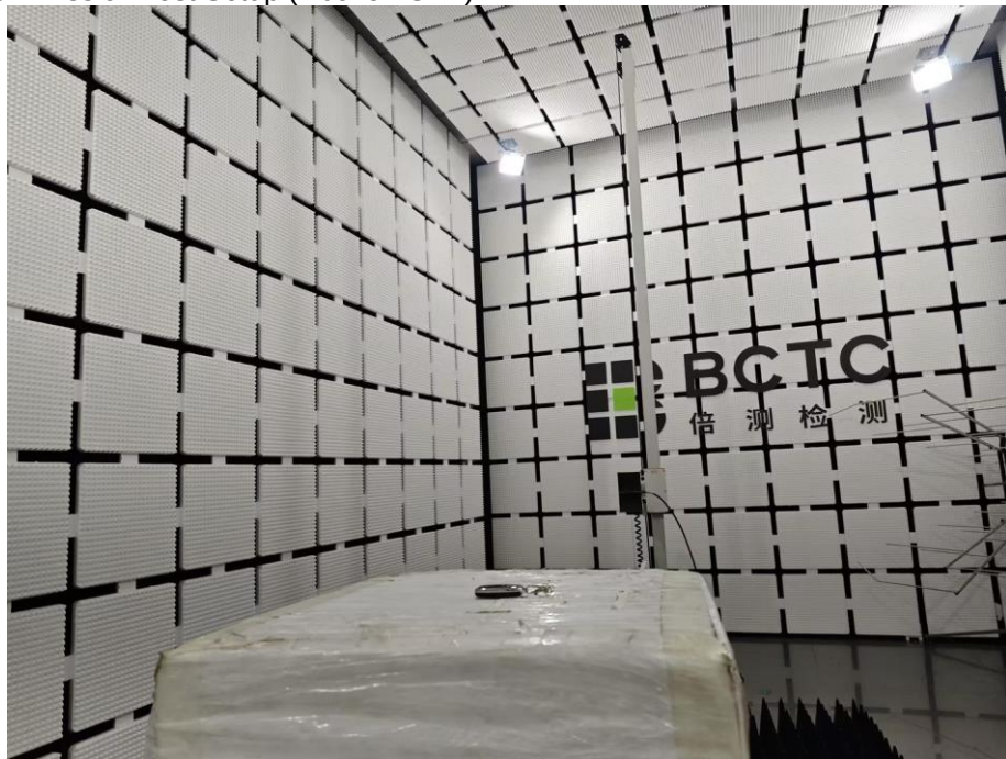
Spurious Emission Test Setup (Above 1GHz)
