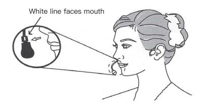
NOTE: Face the white line on themicrophone tip towards your mouth. The amplifier speaker should be atleast 2 feet from the microphone and should face the opposit direction of the white line on the mic tip.
