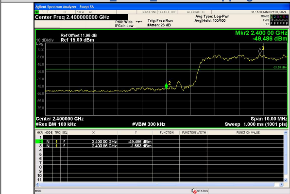
Out Of Band Emission(Left) 8DPSK_3-DH5_Channel Hopping
