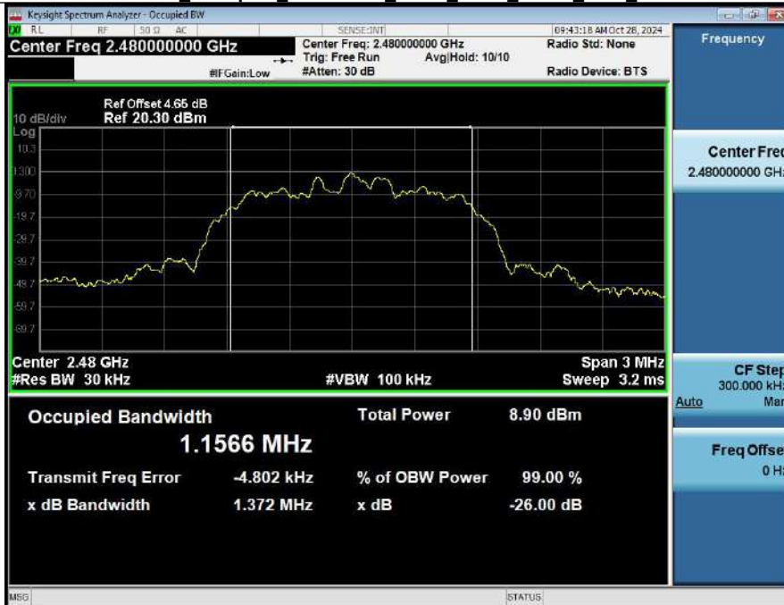
99% Occupied Bandwidth NVNT_ANT1_2-DH1_2480_00
