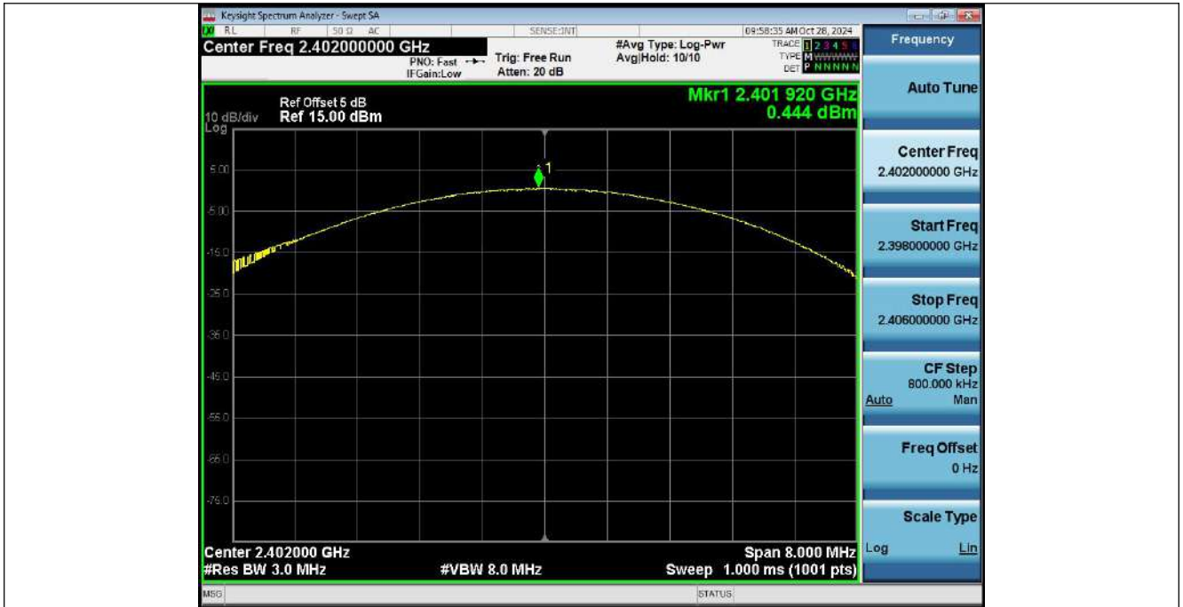
Peak Output Power NVNT_ANT1_3-DH1_2441_00
