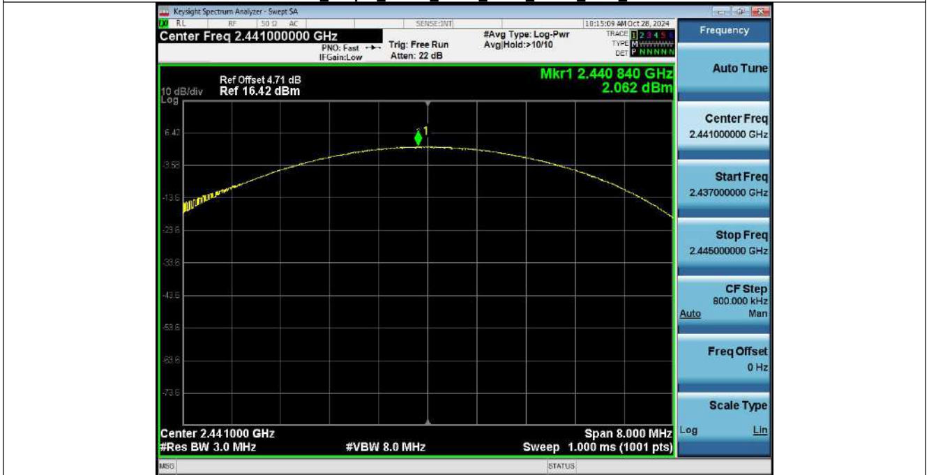
Peak Output Power NVNT_ANT1_3-DH1_2441_00
