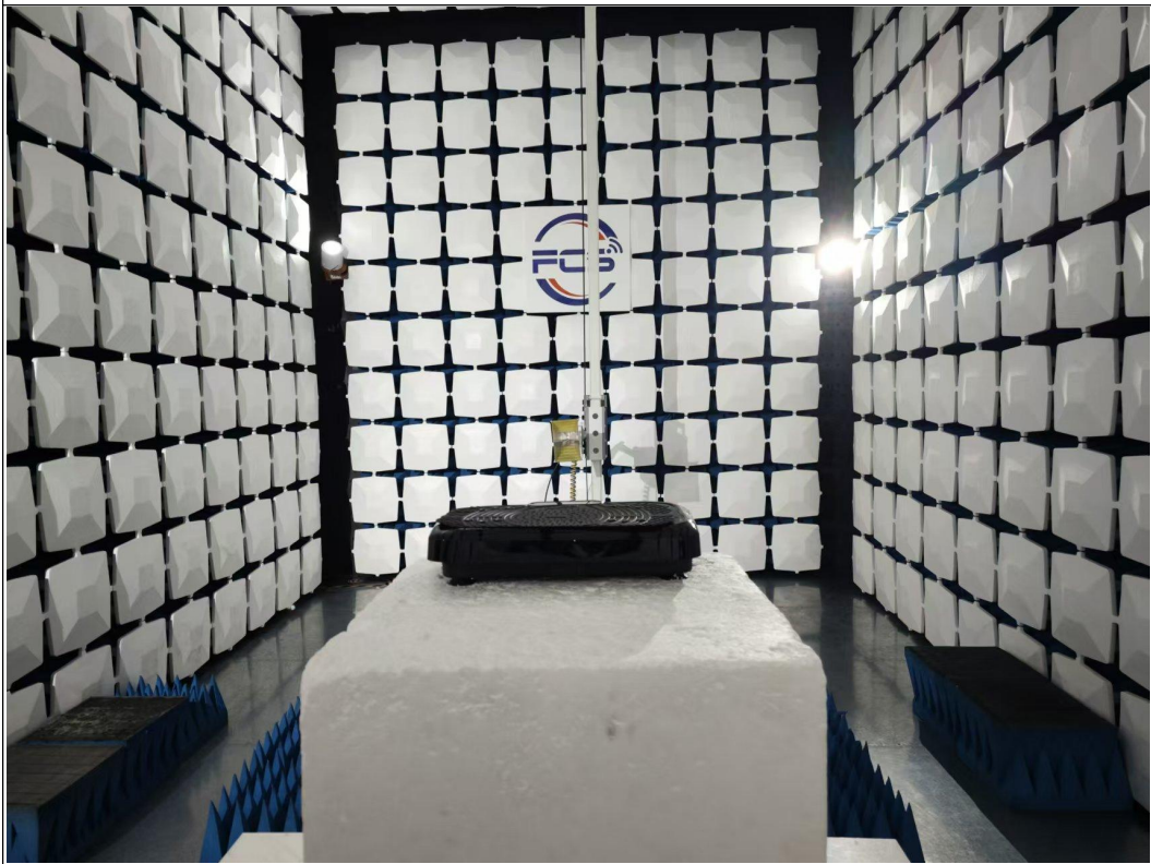
Above 1GHz for radiated emission test setup
