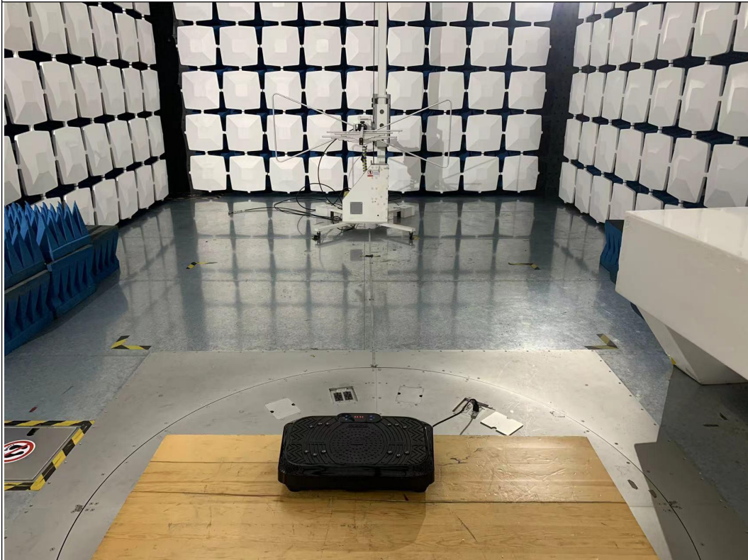
Above 1GHz for radiated emission test setup
