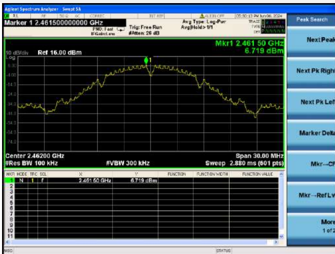
802.11b HIGH CHANNEL, CARRIER LEVEL
