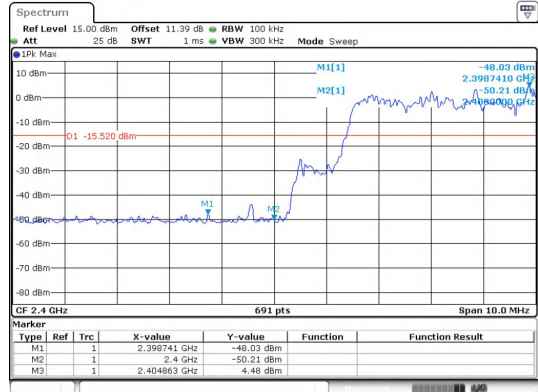
Out Of Band Emission(Left) \pi/4 DQPSK_2-DH5_Channel Hopping
