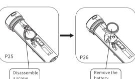
a screw battery Disassemble the battery only when the appliance is being disposed.
