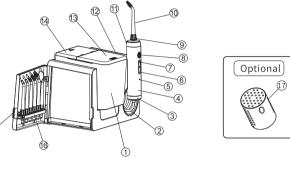
①Reservoir ②Waterhose ③Handle bottom cover ④Handle ⑤Indicator Light ①Tip Eject Button ②Operate Panel ③Reservoir Fixing Plate
