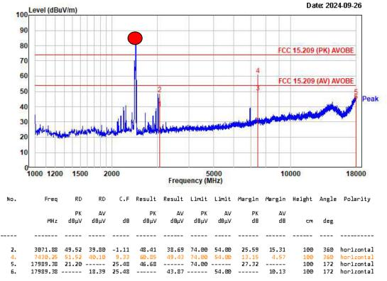
Remarks: C.F (Correction Factor) = Antenna factor + Cable loss - Preamp gain
