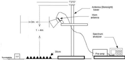
Above 18 GHz shall be extrapolated to the specified distance using an extrapolation factor of 20 dB/decade form 3m to 1m.
