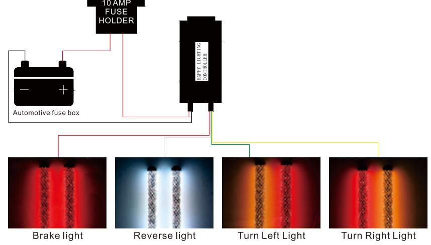
Diagram1: Wiring direct to Automotive fuse box and using APP or RF remote control to turn on/off. Need to add 10AMP fuse on red 12V+ wires.
