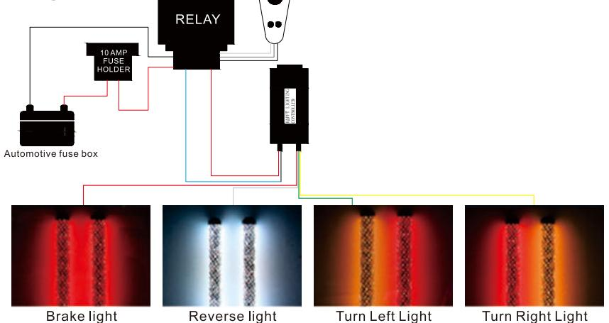
Diagram2: Wiring with a switch. You can add a new dedicated switch or use an existing light switch that outputs 12V+ when ON. You will need to add a 10AMP fuse on the RED 12V+ wire and also requires a 12V relay.
