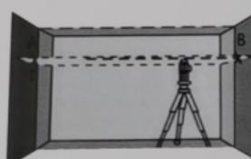
Move the measuring instrument closer to wall B (without rotating the measuring instrument), start the measuring instrument, and level the instrument.Adjust the height of the measuring instrument (with a tripod, if necessary, use the spacer), so that the intersection of the laser lines is accurately projected on point II of wall B.
