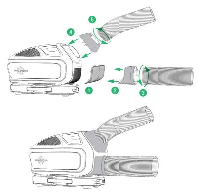
This configuration allows you to place the Mark 3 directly outside the area you are trying to cool and aim both ducts into the space to conserve room.
