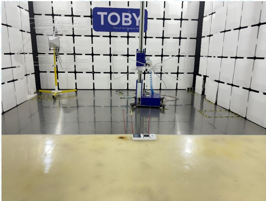
Photo of Setup for Radiated Emission (Above 1 GHz)
