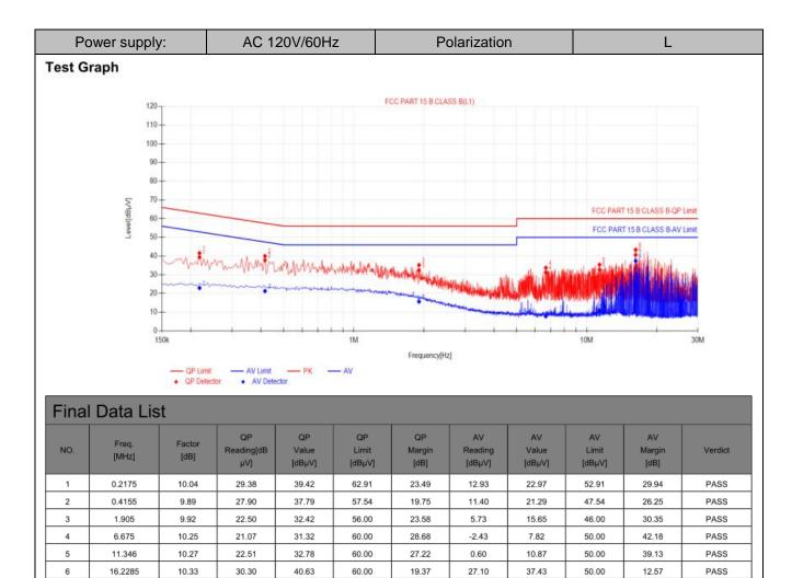
Note:1).QP Value ( $dB\mu V$ )= QP Reading ( $dB\mu V$ )+ Factor (dB)
