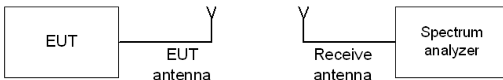
Figure 7.1.1 6 dB bandwidth test setup
