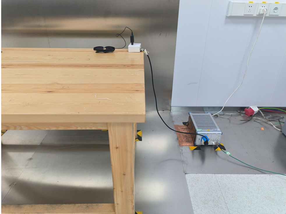
Radiated Emission Test View[(Below 1G)
