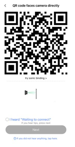
The QR code that appears on the mobile phone is scanned against the camera lens, and the device emits a prompt sound "QR code scan successful" and "WiFi connected", click Next, and wait for the network configuration to be completed.
