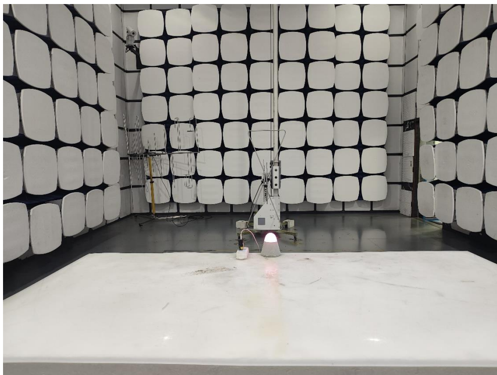
Photo of Radiated Emission test
